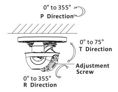
Figure 2-9 3-axis Adjustment
