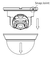
Figure 2-1 Remove the Bubble
