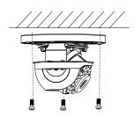
Figure 2-8 Fix the Camera to the Ceiling
