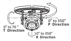
Figure 2-4 3-axis Adjustment
