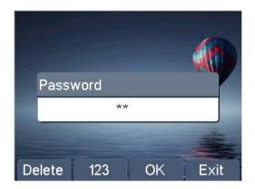
Picture 104 - Phone keypad lock password input interface
