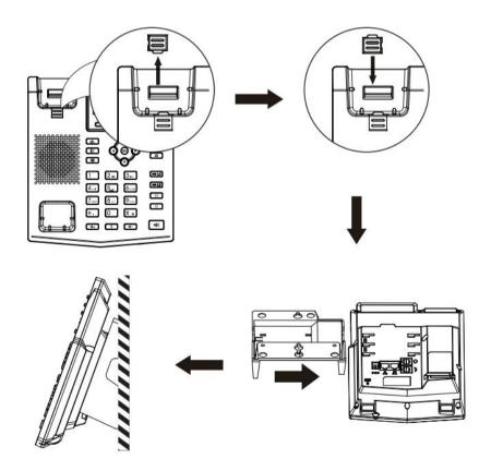
Picture 2 - Wall-mounted installation
