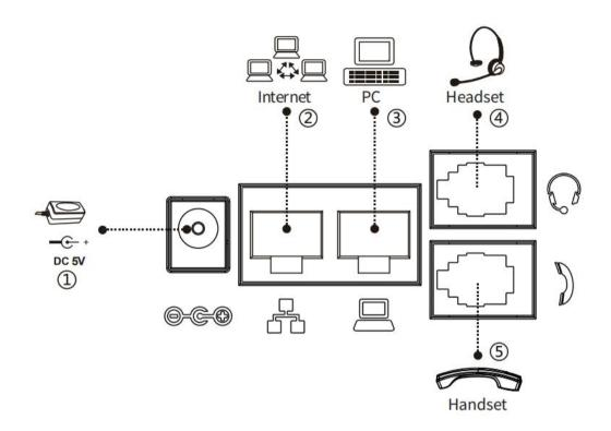
Picture 3 - Connecting to the Device
