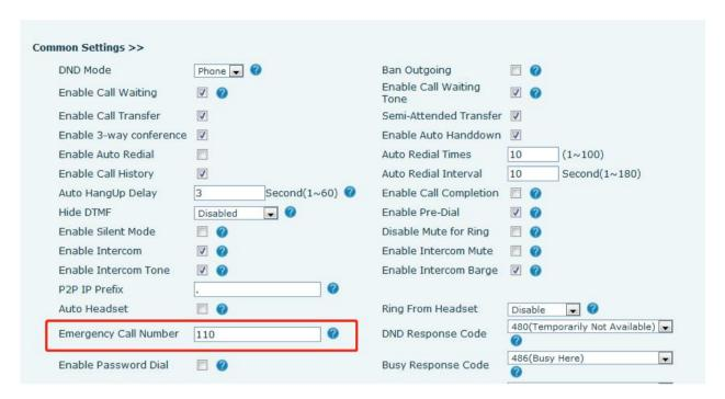
Picture 50 - Set up an emergency call number
