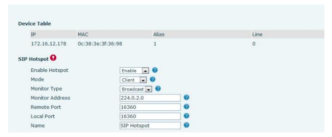
Picture 72 - SIP hotspot client configuration
