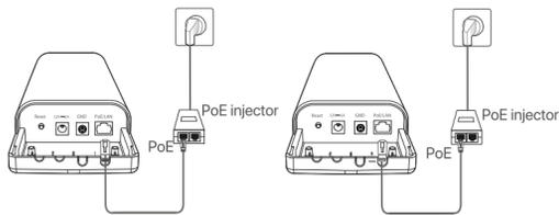
About 1 minute later, when the LED1, LED2 and LED3 indicators of one CPE light solid on and those of the other CPE keep blinking, the automatic bridging succeeds. After the bridging succeeds, the DHCP server of the CPEs will be disabled automatically. The IP address of the CPE working in AP mode remains 192.168.2.1, and the IP address of the CPE working in Client mode is changed into 192.168.2.2.
