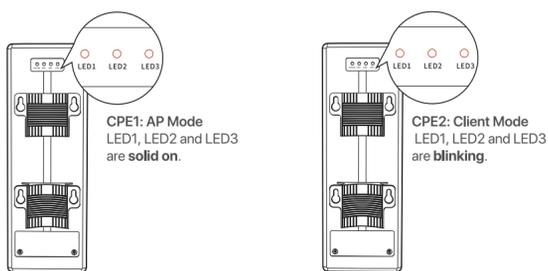
Tips: If the automatic bridging fails, restore the two CPEs to factory settings and try again. Reset method: When the PoE/LAN LED indicator lights solid on or blinks, hold down the Reset button for about 8 seconds and release it when all LED indicators light up. The CPE is restored to factory settings.
