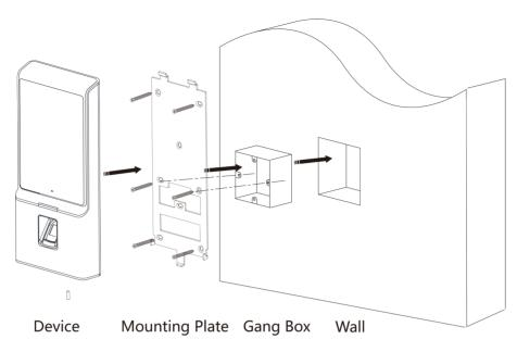
Figure 3-3 Install with Gang Box
