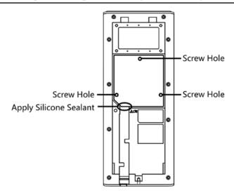
Figure 3-2 Device Back Sheet
