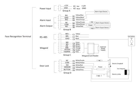
Figure 4-2 Device Wiring
