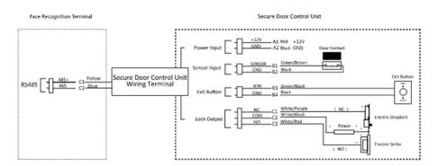
**Figure 4-3 Secure Door Control Unit Wiring**
