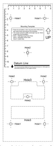
**Figure 3-4 Mounting Template**
