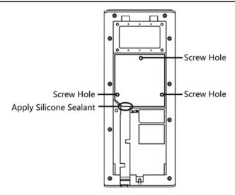
Figure 3-6 Device Back Sheet
