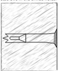
**Figure 3-5 Insert Screw Socket**
